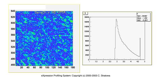
Figure 6: Zoomed image of log intensities and a histogram revealing intensity saturation.
